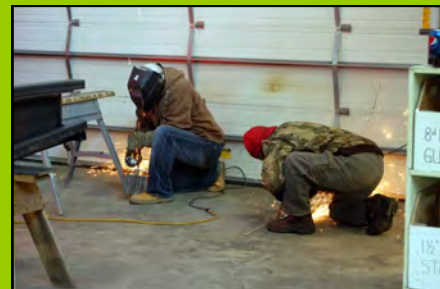
Above: Students use grinders to prepare pieces of metal for further Vertical-Up Shielded Metal Arc Welding (SMAW).
